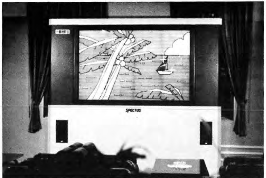
Crystal Color system in a multi-purpose meeting room has 1.2 m x 1.8 m display screen.
